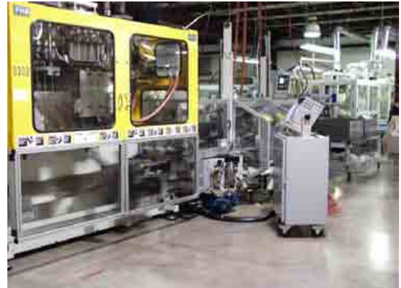
Blow Molding Production for plastic semen tubes Annual capacity: 55mio
